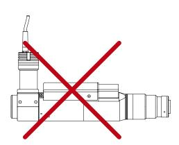
MZMT12X series lenses must be operated according to the drawing above. Only vertical operations are allowed. MZMT12X series lenses might not to work properly or might be permanently damaged if used horizontally.
