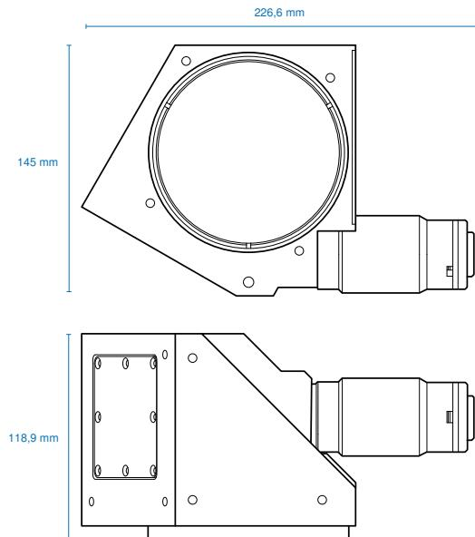
**LTCLHP080-B** Telecentric HP illuminator, beam diameter 100 mm, blue
